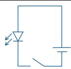
In a simple circuit, the switch is the part of the circuit we control and is our INPUT, and the light is the OUTPUT, (what the circuit does). Even a simple circuit allows us to collect data as in the following table.
