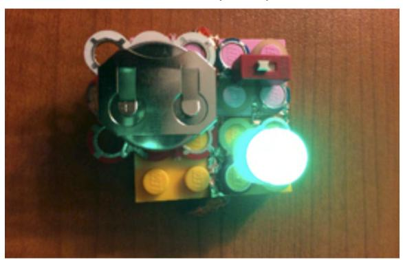
your design, or even put it inside, it can shake the whole structure. In the top photos, a tiny circuit was assembled using copper tape on LEGO bricks. Try adding a motor and putting the circuit into a paper box to make a moving creature! You can also embed the circuits on a cork, pins and pipe cleaners. Take a look at the <a href="https://www.lectrify.it/projects">www.lectrify.it/projects</a> for more ideas!
