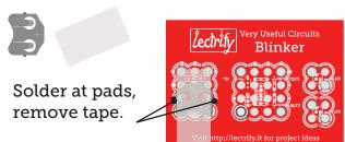
Step 2: Insert Components and solder from back of board
