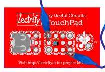
Clip each touchpad on board to aluminum foil and place side by side. Place fruit on foil touching both pieces of foil.
